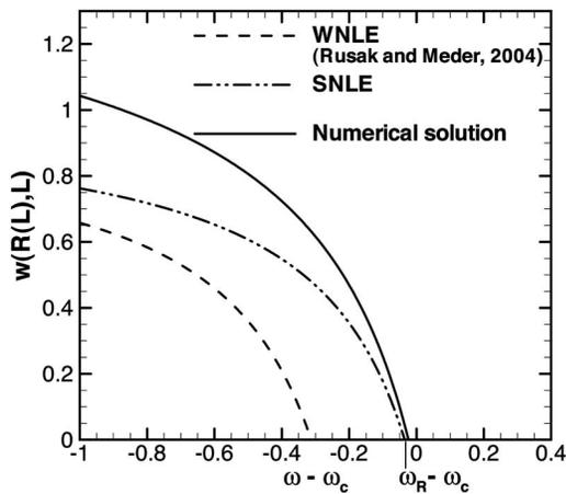
FIG. 1. Axial velocity  $w[R(L), L]$  at the exit plane wall of a weakly contracting duct with  $L=1$ ,  $R(L)=0.9$  ( $\epsilon=0.1$ ). Comparison of the present strongly nonlinear expansion (SNLE) with the weakly nonlinear expansion (WNLE) of Rusak and Meder (Ref. 2) and with the numerical solution.
