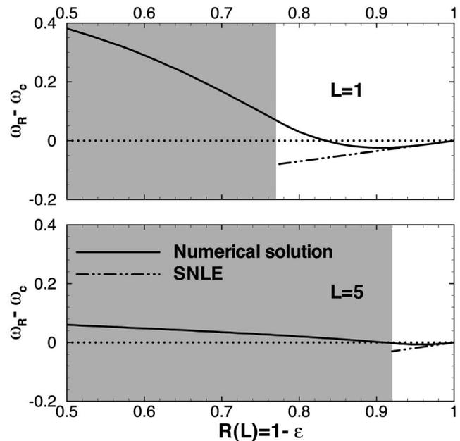
FIG. 2. Value of  $\omega_R - \omega_c$  ( $\omega_R$  being the swirl at which a wall recirculation is obtained) as a function of the exit duct radius  $R(L)$ , for  $L=1$  and  $L=5$ . Comparison between the SNLE [valid in the vicinity of  $R(L)=1$ ] and the numerical solution. In the shaded region, the recirculation is obtained for  $z < L$ , inside the duct.
