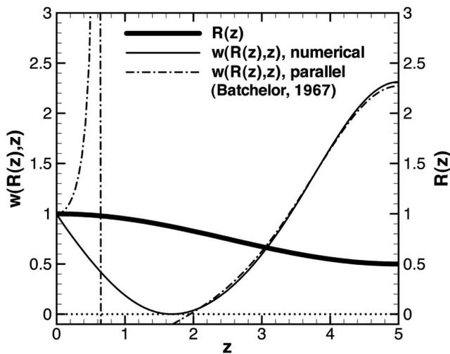
FIG. 3. Axial velocity  $w[R(z), z]$  at the wall of a contracting duct with  $L=5$ ,  $R(L)=0.5$ , in a situation of incipient recirculation ( $\omega - \omega_c = \omega_R - \omega_c = 0.0594$ ). Comparison of the numerical solution with the parallel approximation of Batchelor (Ref. 4).
