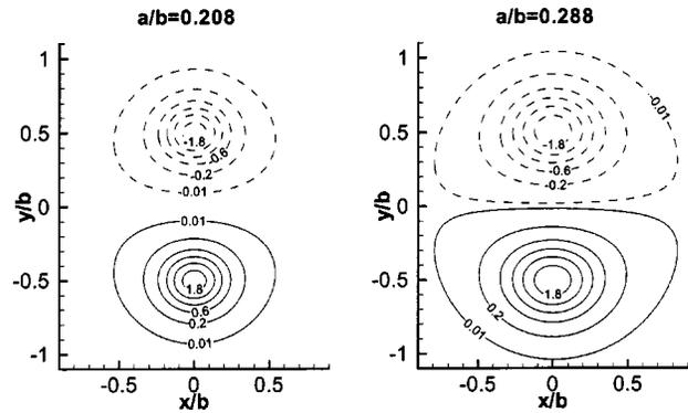
FIG. 1. Vorticity distributions of the dipoles for  $a/b=0.208, 0.288$ . The isolevels represent the vorticity  $W_L 2\pi a^2/\Gamma$ . Dashed lines represent negative values. These dipoles are steady solutions of the Euler equations (see Ref. 1).
